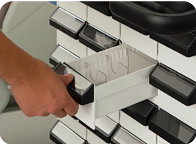
SmartCart assigns a medication bin for each patient, opens bin for nurse to place all medications
